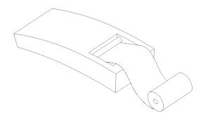
Put the paper roll at the back of the device ( See draw) Introduce the paper under the cylindrical paper driver. Maintain a light pressure on the paper, press the paper feed (-). Ensure you a good guidance of the paper. Put the paper roll in its compartment and strongly push it downwards. You will feel a click as soon as the paper roll will finds its housing.
